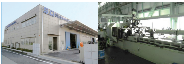
The friction welding machine at Shiga plant responds to large prototype parts.
